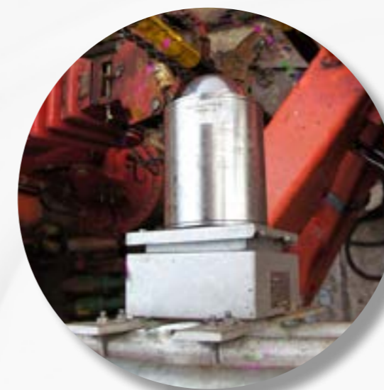
1. DATAEAGLE at the fixed side in the Ex-protective housing.
