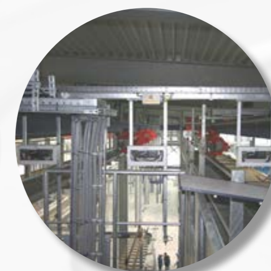
2. DATAEAGLE is located directly in the ceiling construction and is the base station (Master).
