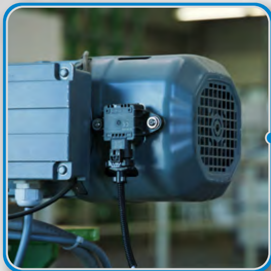
DATAEAGLE Condition Monitoring System (CMS) direkt am Motor
