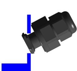
Fig. 1 - threading in the cable screw connection
